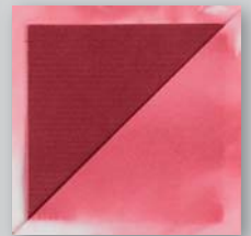
Normal boards bleed out if they are exposed to moisture.
